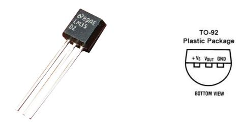
The LM35 will need power supply, +Vs from 4V to 20V. We can use +V pin from 3.5mm Jack directly.
