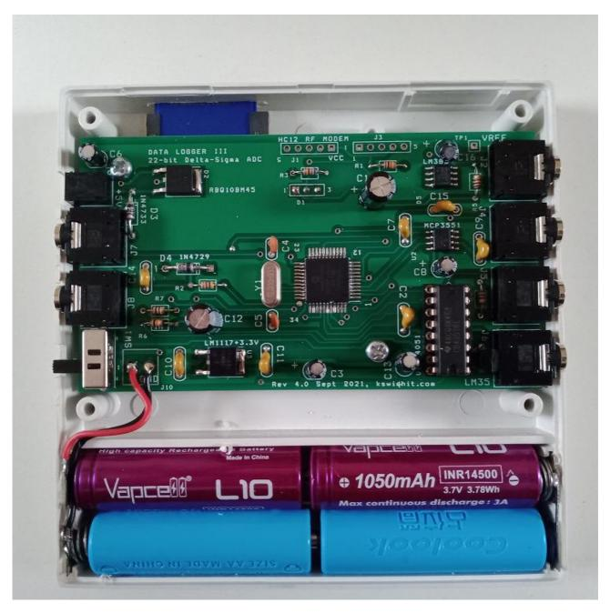
The AA size (14500) rechargeable Lithium ion battery is best for mobile operation. No need external power.
