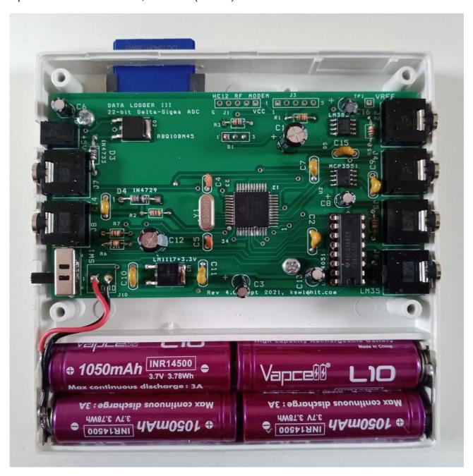
For sensors that need higher voltage, we can use Four Cells series connected +14.8V as well.
