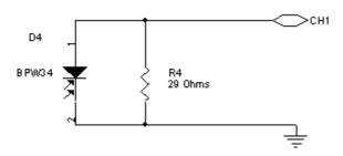
The voltage developed on the load can tie to the input of the data logger directly, no need amplification.
